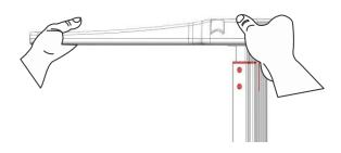
1. Place both hands in place as figure to hold the height rod's head.
