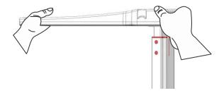
2. Place both hands in place as figure and open the height rod's head.
