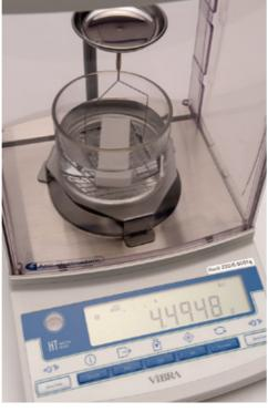
VIBRA HT series has Se-CAL function as standard. In Se-CAL, the balance can perform self-calibration fully automatically according to pre-installed
